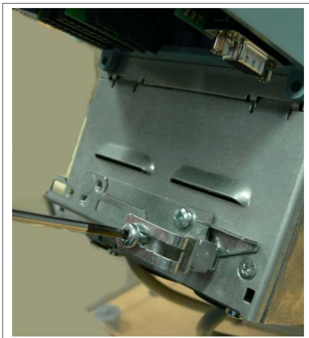
Figure 4-13. Remove the screw of the grounding clamp
